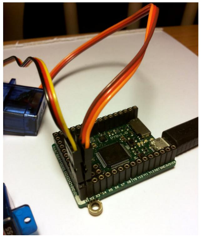
In this picture there are male-male double adaptors to connect the servos to the header pins on the pyboard.
