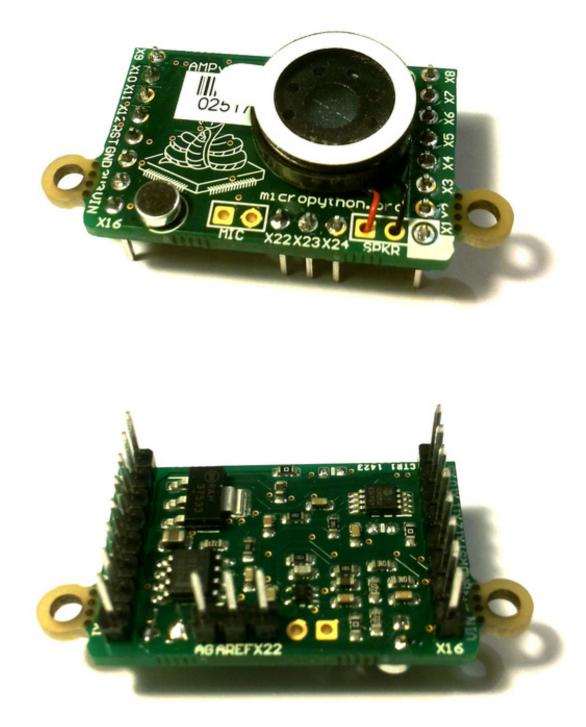
The following video shows how to solder the headers, microphone and speaker onto the AMP skin.
